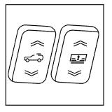
The sunroof/sunshade switches are located in the headliner between the driver and front passenger.
